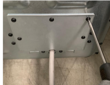
Assemble cover and tighten screws.
