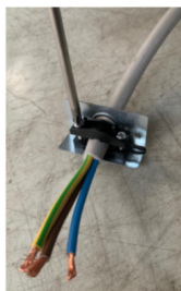
Fix power cord to the plastic holder.
