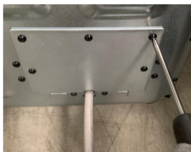
Assemble cover and tighten screws.
